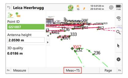
Pressing **(F4) Meas+TS** initiates the GS measurement and then, once stored, automatically initiates the TS measurement.
